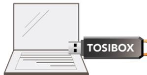
2. Open the TOSIBOX® Key software by plugging a matched Key into the USB port of your computer.
