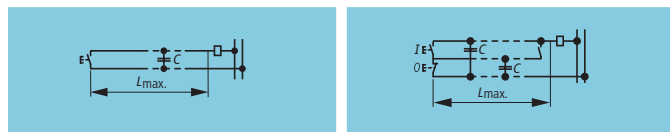
Figure 46: Two-wire control (left) and three-wire (pulsed) control
