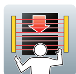
Monitoring open hazardous area with light curtain
