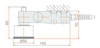
Protects load cell against lateral loads. Used in accurate and vibrating weighing systems.
