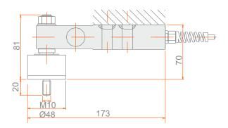
Protects load cell against lateral loads. Used in accurate and vibrating weighing systems.
